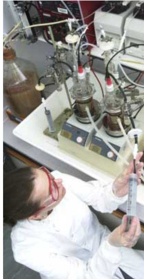
Industrial biofilm generator at NCIMB
